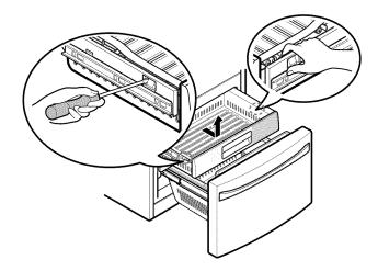
2. To replace, slightly tilt up the front of the drawer, insert drawer into the frame, and push drawer back into place until you hear a click.
